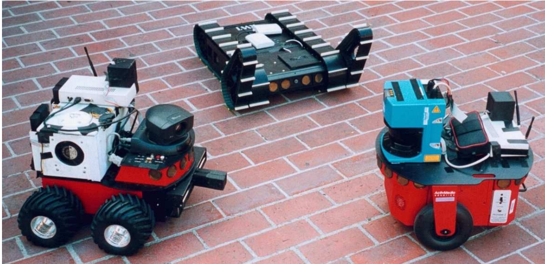
Figure 1. Pioneer-1 AT (left), RWI Urban Robot (middle), and Pioneer-2 DX (right) platforms
